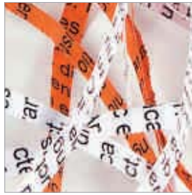
Security level 2 · Strip cut Shredding no. 5 3.9 mm
