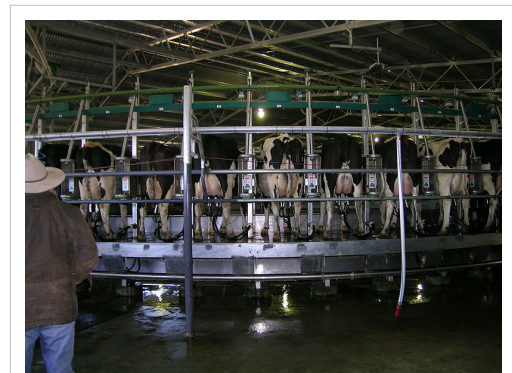
An 80-stand rotary dairy that is fully computerised and records milk production.
