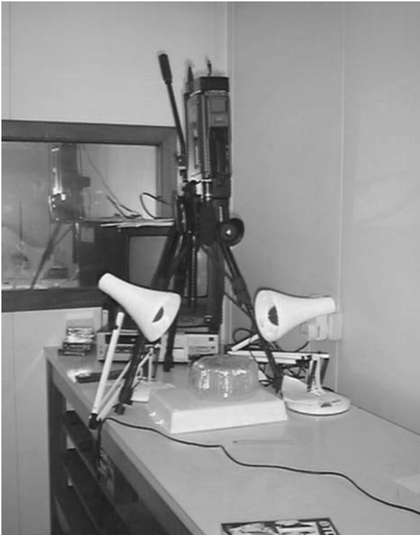
Fig. 2. Arena in position for filming showing the camera, red lights and time lapse recorder.
