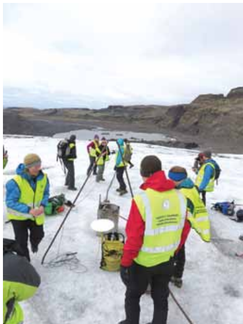
Students in the glaciology course at University of Iceland install an ablation wire in the surface of Sólheimajökull Glacier with a steam drill. The wire ablates out of the ice during the summer providing information about the rate of ice melt. GPS instruments are used to measure the location of the site and track the velocity of the glacier.
