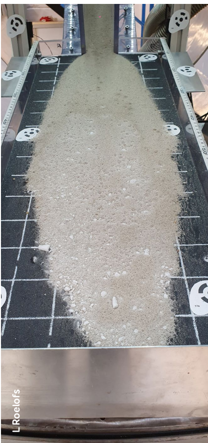
The mixture of sediment and carbon dioxide ice flows down the slope under martian conditions in the chamber.
