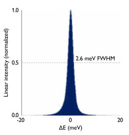
Zero loss peak: Nion HERMES at 20 kV with Nion IRIS EELS, 1000 spectra of 3 ms, aligned.
