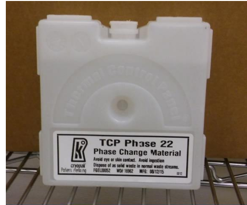
Figure 17: Thermal block used to keep a constant temperature in the ice chest
