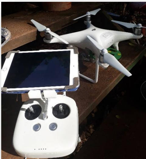
Figure 3. DJI Phantom 4 Advanced with attached RGB and MAPIR Near Infrared Cameras.
