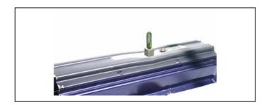
The bodywork dent is reshaped by turning the hexagon bolt (anticlockwise) on the dent removal fixture.
