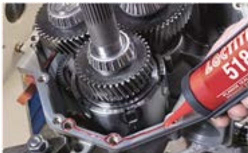
Fig. 5.17 Application of an anaerobic product to a flange.
