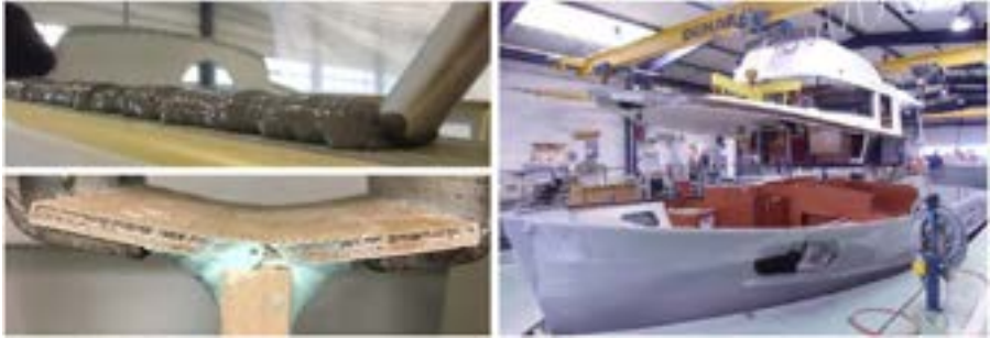
Fig. 3.17 Selected applications in the marine industry: deck-to-hull and bulkhead bonding by 2C PUR adhesives.
