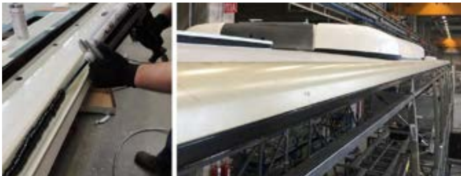
Fig. 3.19 Example of modular assembly in bus manufacturing [13]: a prefabricated roof is bonded to the bus chassis by 2C PUR.
