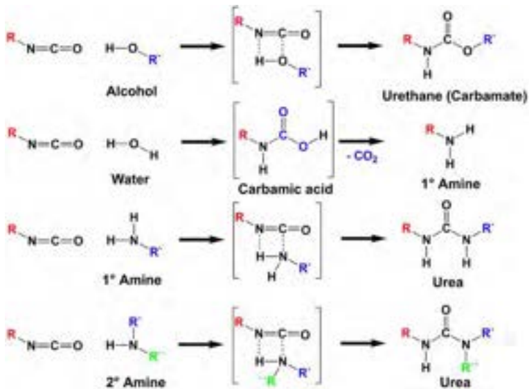
Fig. 3.8 Set of basic isocyanate-related chemical reactions including possible transition states used in 1C and 2C PUR adhesives. Courtesy of Sika Technology AG.
