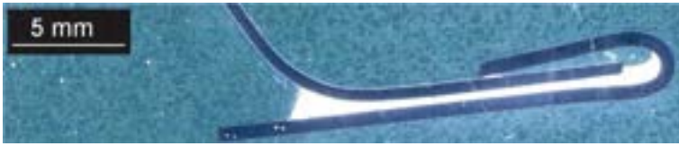
Image 2.5 Typical hem flange cross-section with LORD Versilok adhesive.
