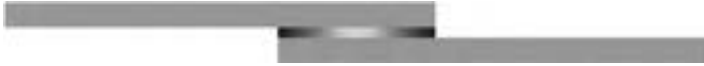
Fig. 33.12 Schematic concept of the functionally graded joints obtained by induction heating, with the smooth variation of the properties of the adhesive layer being represented by a gradient.
