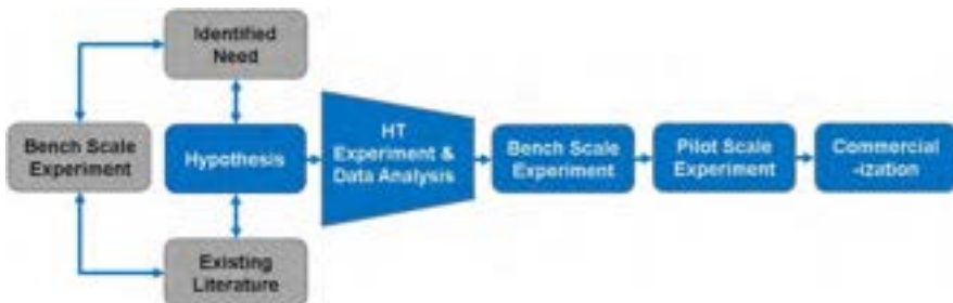
Fig. 22.1 R&D process flow showing the place of HT in the overall work process [10,13–17].
