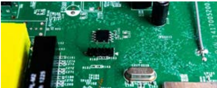
Fig. 9.1 Dewetting of a substrate (in this case a circuit board) by a liquid (a conformal coating).
