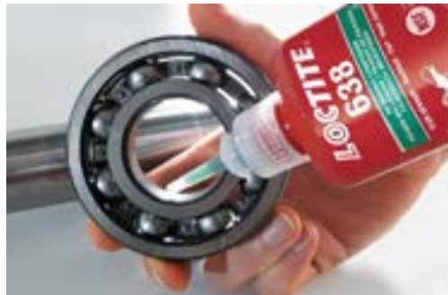
Fig. 5.16 Application of an anaerobic retaining compound to a bearing.
