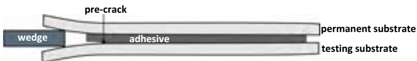
Fig. 22.9 Edge view of a representative wedge test sample to evaluate adhesion durability.
