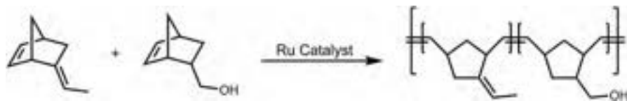
Fig. 7.14 Copolymerization of 5-methanol-2-norbornene (NBOH) and 5-ethylidene-2-norbornene (ENB) by ROMP to study effects of polar functionality on mechanical response. Reproduced with permission from J.M. Dennis, T.R. Long, A. Krishnamurthy, N.T. Tran, B.A. Patterson, C.E. Busch, K.A. Masser, J.L. Lenhart, D.B. Knorr, Influence of hydroxyl group concentration on mechanical properties and impact resistance of ROMP copolymers, ACS Appl. Polym. Mater. 2(6) (2020) 2414–2425. https://doi.org/10.1021/acsapm.0c00352 .
