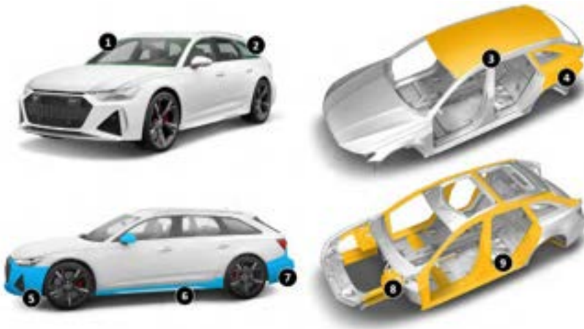
Fig. 26.6 Common repair applications with structural adhesives in damaged light vehicles: (1) direct glazing of windshield; (2) bonding of side windows; (3) bonding of steel roof panel; (4) bonding of steel body quarters; (5) rebuild of plastic front bumper; (6) rebuild of plastic rocker panels; (7) rebuild of plastic rear bumper; (8) reinforcement of steel front side body frame; (9) reinforcement of steel pillars and central body frame components. Credit: Henkel, Adhesive Technologies, www.henkel.com .
