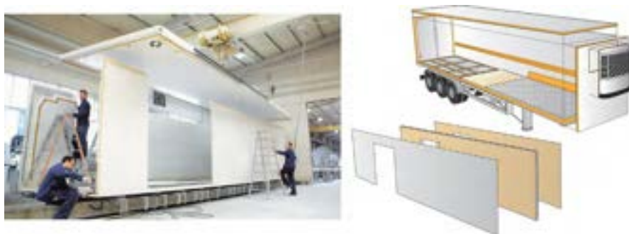
Fig. 3.16 Selected applications in vehicle manufacturing: 2C PUR is regularly employed for sandwich panel fabrication and the assembly of refrigerated trucks.
