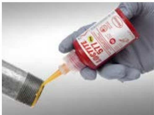
Fig. 5.15 Application of an anaerobic thread sealant to a threaded pipe fitting.
