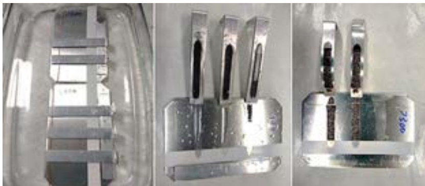
Fig. 22.12 (Left) Example of high-throughput wedge samples submerged in water; (Center) Example of adhesive failure across most of the bondline for an adhesive exposed to mechanical strain and water exposure; (Right) Example of cohesive failure after opening the sample following water submersion.
