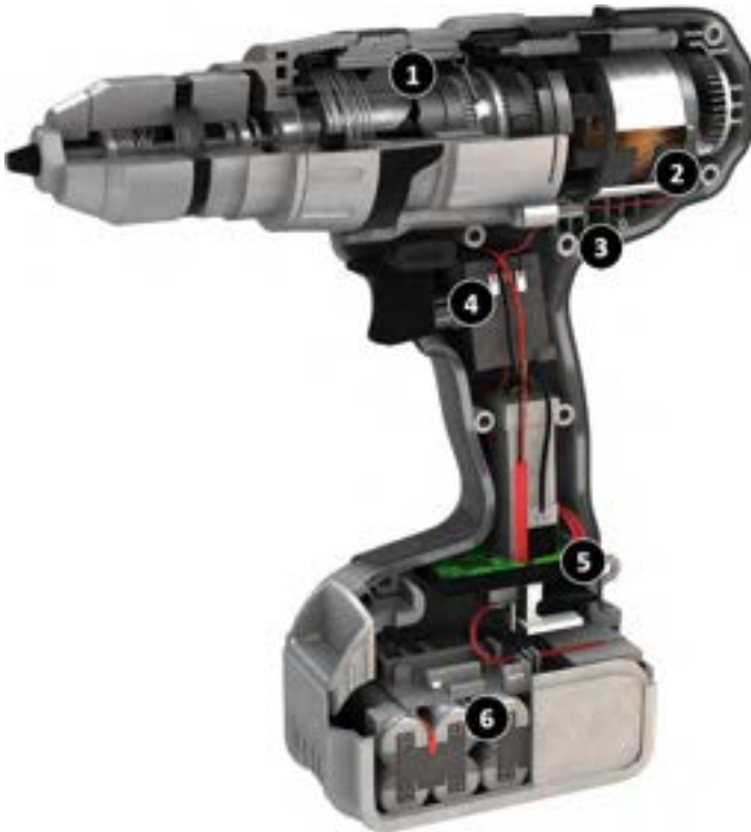
Fig. 26.8 Common engineering adhesive manufacturing applications for a power tool: (1) retaining of gears and bearings; (2) threadlocking of mechanical fasteners; (3) bonding and sealing of enclosure; (4) tacking of electrical connections; (5) assembly and encapsulation of electronics; (6) thermally conductive gap filling of battery cells. Credit: Henkel, Adhesive Technologies, www.henkel.com .
