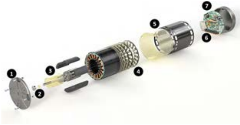
Fig. 26.7 Common engineering adhesive manufacturing applications in electric motors: (1) threadlocking of mechanical fasteners; (2) retaining of bearings; (3) bonding of magnets; (4) bonding of lamination stacks; (5) retaining of stator; (6) thermally conductive bonding of electronics heat sink; (7) assembly and encapsulation of electronics. Credit: Henkel, Adhesive Technologies, www.henkel.com .
