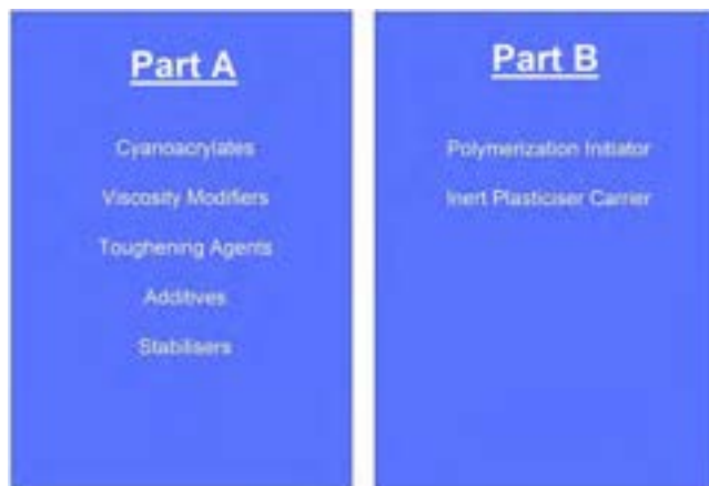
Fig. 4.7 Part A and Part B components in a 2K adhesive.
