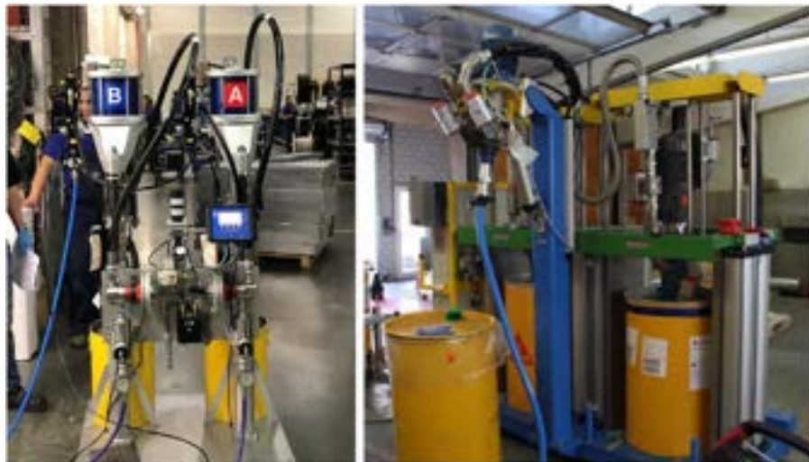
Fig. 3.21 Examples of adhesive dosing equipment. Photo courtesy of Sika AG.
