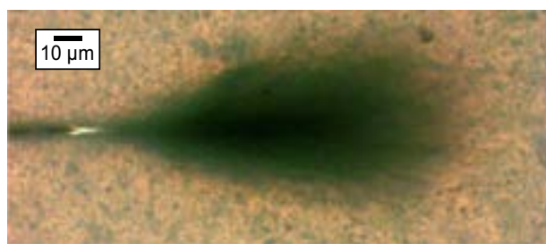
Fig. 8.3 Transmission optical micrograph of a subcritically loaded crack tip in the plane strain region of a 10 wt% CSR-modified epoxy polymer [31].
