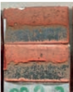
iv) Self-Assembling Monolayer (SAM) did not fail after 49 cycles. Sample pulled on load frame to observe failure mode
