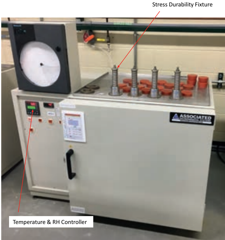
Fig. 24.4 Humidity cabinet loaded with stress durability fixtures.
