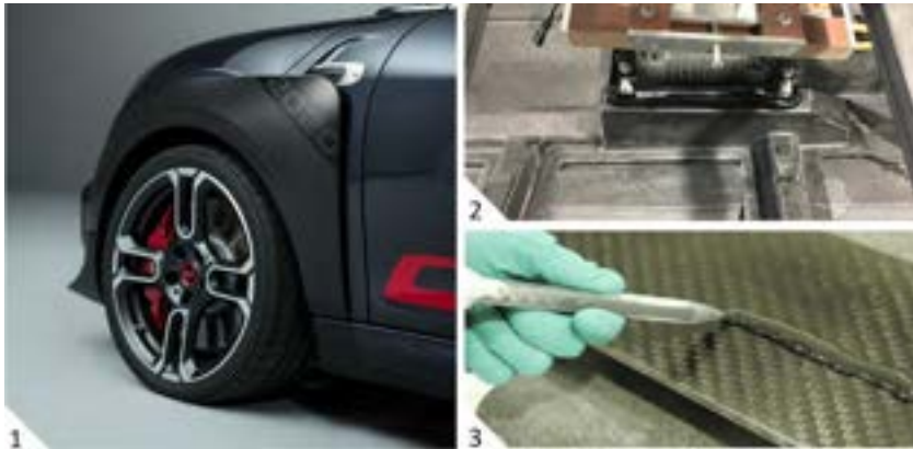
Fig. 3.18 Examples of CFRP components that are assembled using 2C PUR adhesives.
