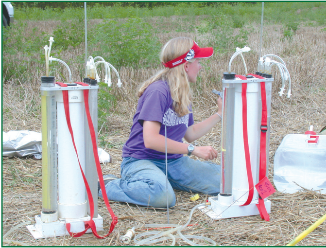
Figure 6. Purdue University graduate student Jenny Krenz records water level measurements from Amoozemeters, which measure hydraulic conductivity in the field using the constant head permeameter method.
