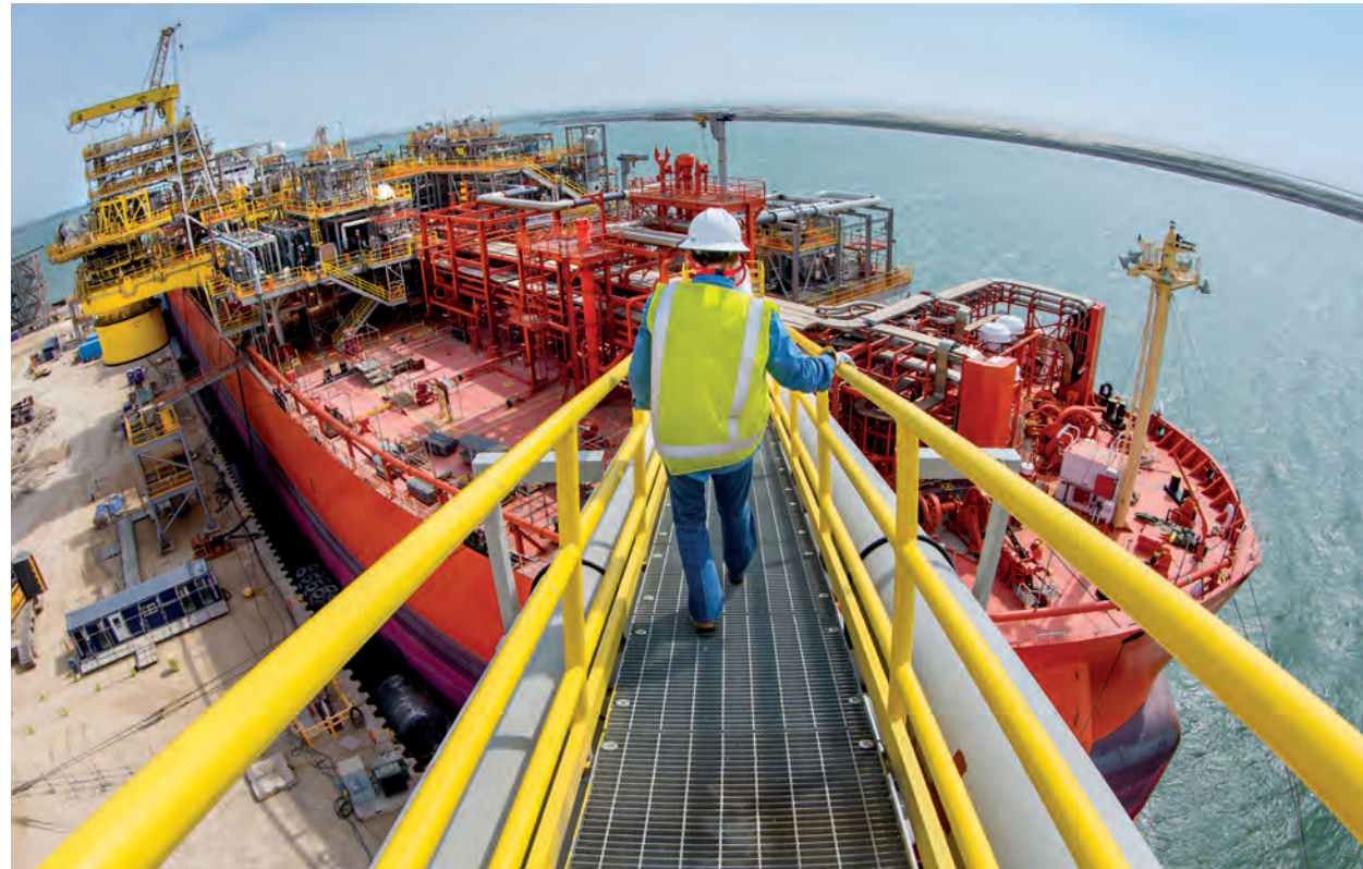
A worker approaches one of the MWCC's rapid-response vessels that can be deployed to capture, process, store and offload liquids during a subsea incident.
