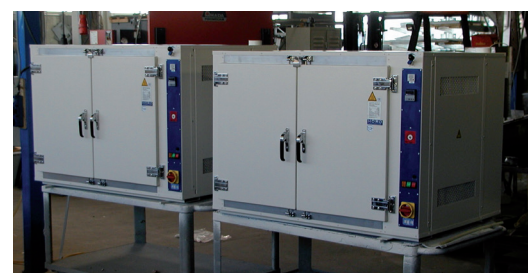
Regeneration of activated carbon filters
