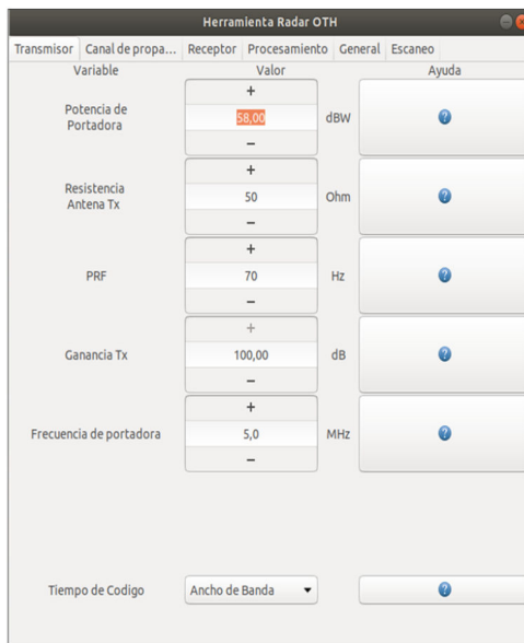
Fig. 7 Second user interface that will generate the transmitted signal, synthesise the received signal, and process it, using input parameters obtained from the first interphase
