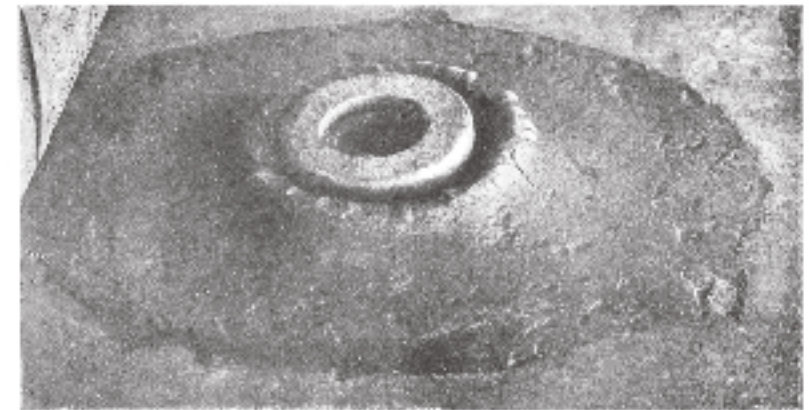
Permanent Splashes left where a Projectile has entered an Armour-plate.
