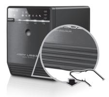
To take the HDD out from the device, slightly press down the handle and pull it out.
