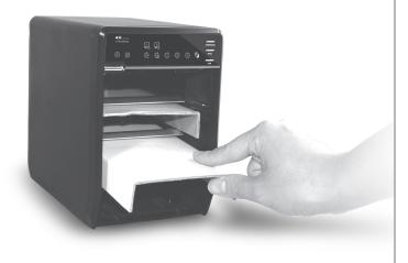
Slide 4 HDDs into the chassis and make sure they are securely installed in order from up to down.
