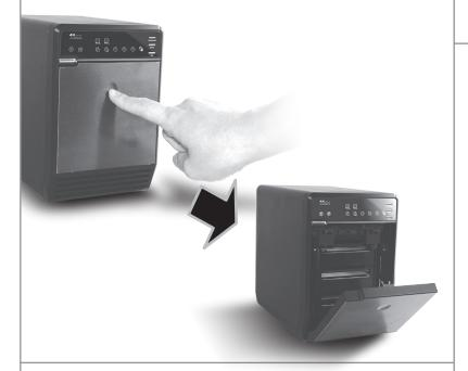
Press down the rib to detach the metal frame and remove it.
