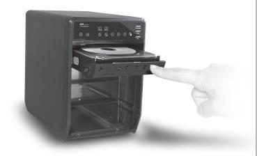
NOTE: Make sure the HDD1 is securely installed in slot 1. Otherwise the PC may not recognize the device. The content of slot 2 - 4 may very.
