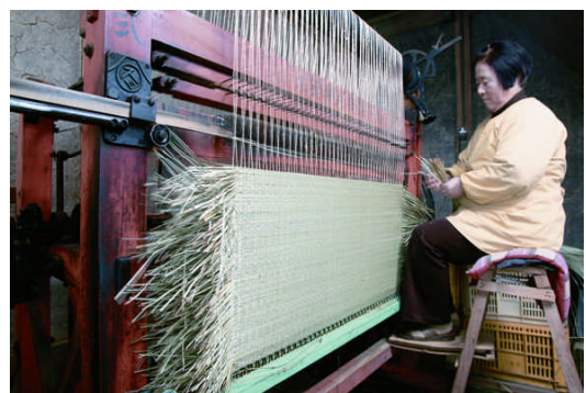
Fig17: Manufacturing process of Shichitoui tatami-omote(surface of tatami)
