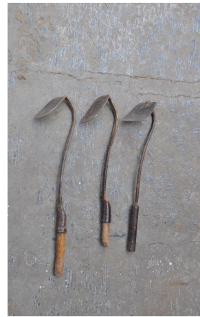
Juetou (used in digging soil and rocks)
