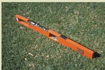
Electromagnetic sensor (EM38 by Geonics Limited) used to remotely measure the apparent or bulk electrical conductivity (ECa) of the soil. Photo by B. Hanson, University of California, Davis, 2000. ©University of California.
