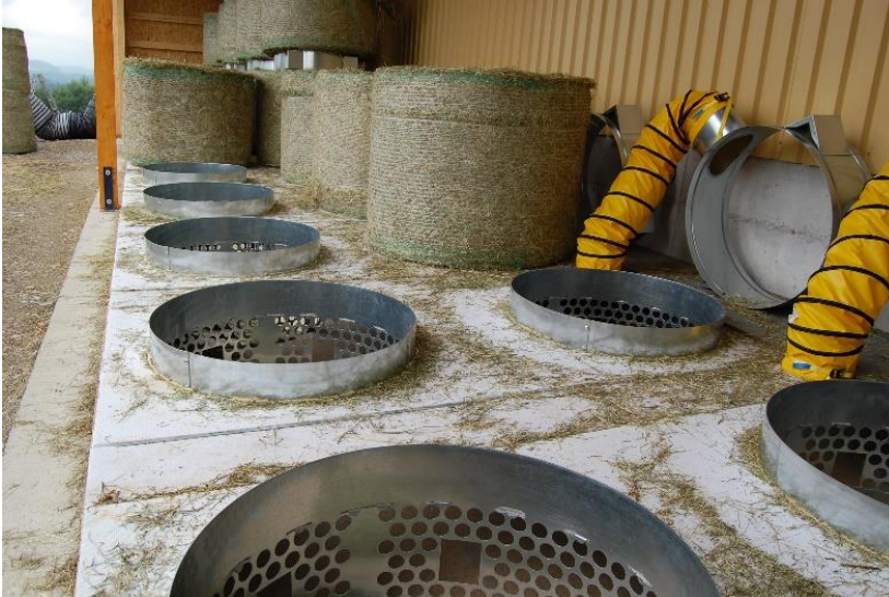
Figure 57 In bale drying, the moist hay is pressed into bales and the bales are aerated.
