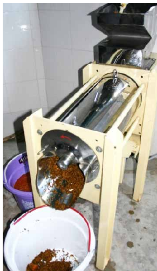
Figure 13 Seed separator (Photos: A. Ait-Hamou)
