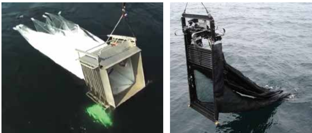
Figure 6. Multiple net systems. Left, MultiNet sampler and right, MOCNESS net
