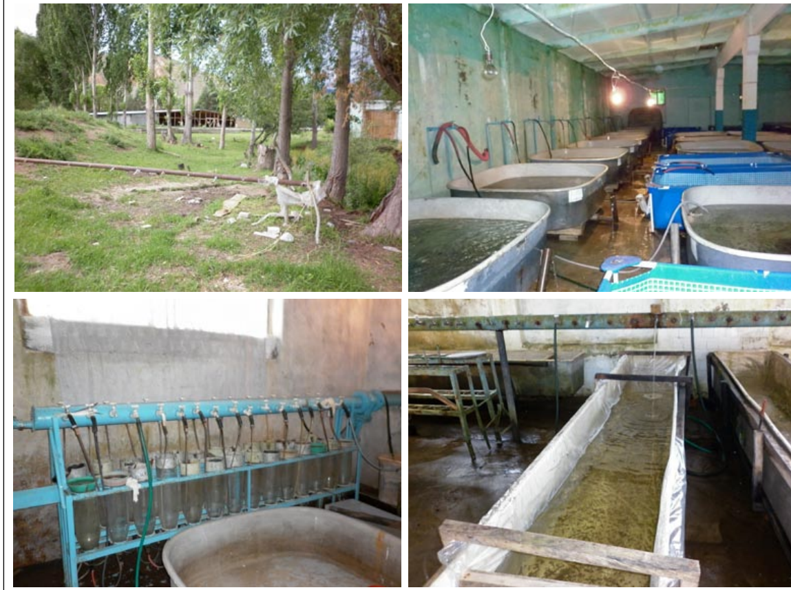
PLATE 4 Provisional pipe supplying water for incubation of carp eggs (top left) and tanks for rearing trout fry and fingerling in Ton fish Hatchery (top right). Zuger jars and larvae rearing tanks in Karakol Fish Hatchery (bottom)
