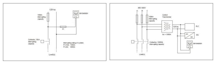
Figure 1 Overall interrupting rating based on F1 (5000A max.)
