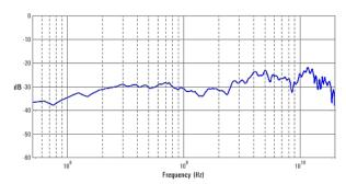
Common mode rejection ratio of 1169A
