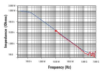
Input impedance over frequency (Red = measured, Blue = model)
