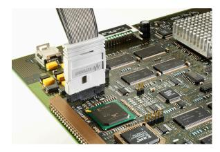
E5346A 34-channel Mictor connector probe
