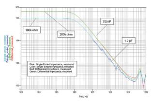
V<sub>out</sub>/V<sub>in</sub> frequency response of N2752A (at 2:1) with browser tip
