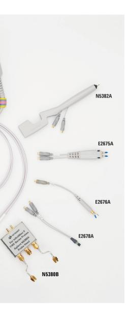
**N5380B 13-GHz high-bandwidth differential SMA** probe head provides maximum bandwidth for SMA-fixtured differential pairs.
