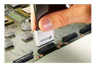
E5385A 34-channel Samtec connector probe
