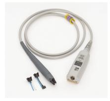
The N2750A Series InfiniiMode differential probes are a new generation of low-cost, 1.5 GHz, 3.5 GHz, and 6 GHz differential active probes compatible with Infiniium oscilloscope's AutoProbe interface.
