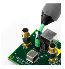
N2750A with N4822A socketed tip for application fixtures
