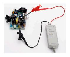
N2790A measuring a power supply signal
