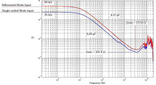
Probe input impedance vs. frequency
