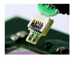
N2887A InfiniiMax Soft touch Pro Probe Adapter adapts from the Keysight Pro Series (36 ch) Soft touch connectorless logic analyzer foot print to the Keysight InfiniiMax I & II series probe amplifier input connectors
