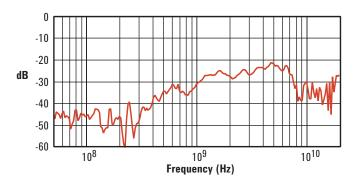
Common mode rejection versus frequency.
