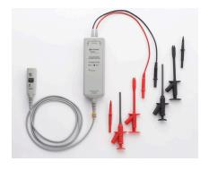
N2790A 100 MHz high voltage differential probe
