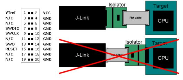
The Emulator side of the Isolator is plugged directly into the Emulator. The Target side is connected to the target via a 20-pin flat cable.
