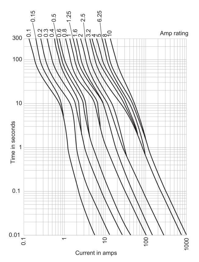
LPS-RK\_SP 600Vac/300Vdc, 1/10-60A dual element, time-delay fuses
