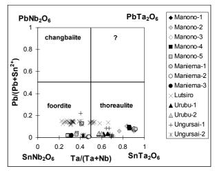
FIGURE 1. The foordite-thoreaulite-changbaiite-PbTa $_2O_6$  quadrilateral diagram (atomic proportions), showing considerably limited solid solution of the Pb-based components in foordite-thoreaulite.
