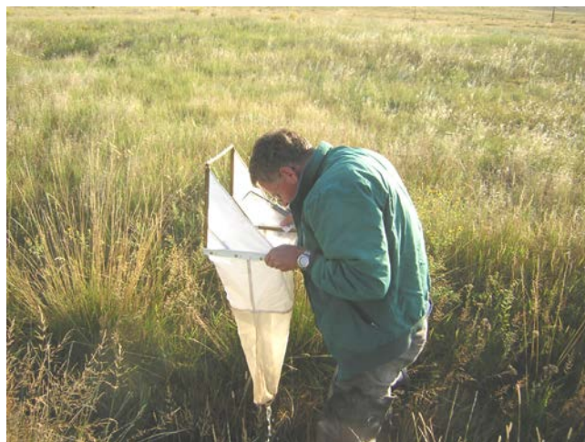
Figure 8. Surber sampler showing capture net and frame, Graves Creek, Soapstone Prairie Natural Area, Larimer Co., Colorado.
