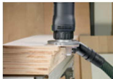
Chamfering plastic or solid wood veneer.
