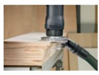
Chamfering plastic or solid wood veneer.
