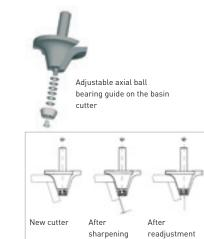
sharpening with offset to ball bearing guide readjustment
