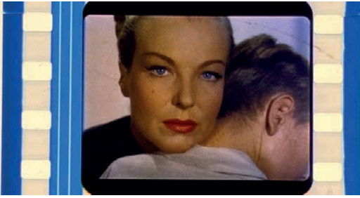
Fig.14. GEM SUPERcineCOLOR print with false coloration giving magenta cast to both neutrals and shadows.
