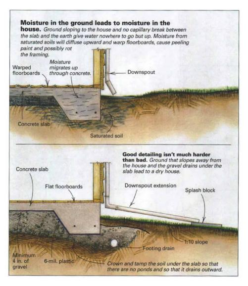
consisting of solid pipe leading to daylight. If you use pipe (as opposed to just gravel) in a footing drain, it should be slightly pitched toward the outlet, or at least not pitched backward. It should have surface clean-outs every 50 ft. Discharge by gravity flow is preferable to a sump pump. Sump pumps are a weak link, likely to fail when most needed, but a gravity drain may not be possible if the footing drains are deeper than any possible discharge point.
