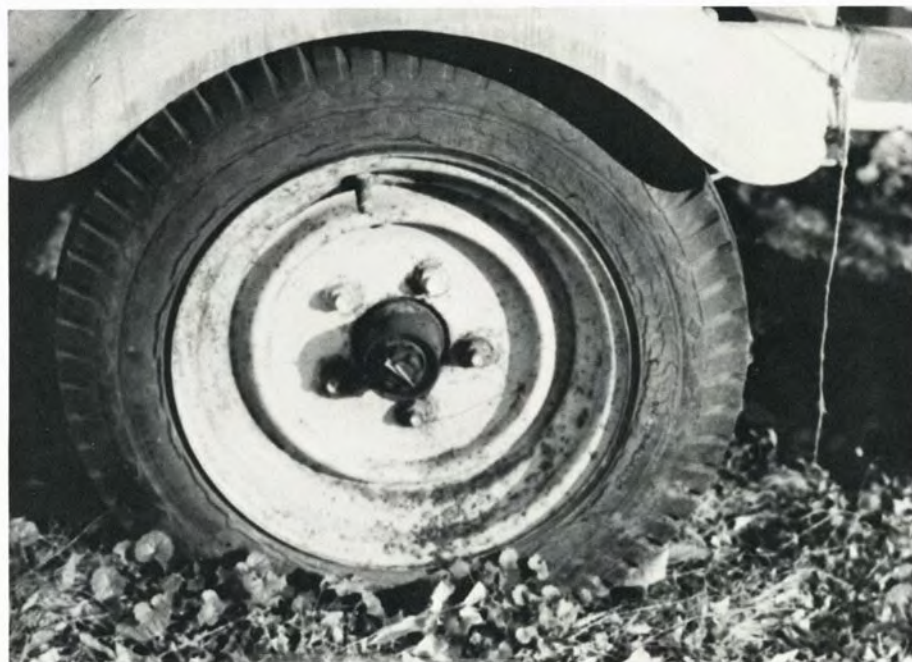
Above, look over your tires. Cracks along the tire's sidewall, as shown here, are a sure sign of fatigue. Time to replace this tire.
