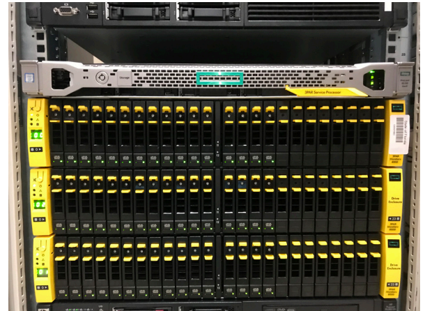
New Storage Area Network (SAN) increases the courts system’s highly available and redundant data storage capacity by approximately 90 Terabytes.
