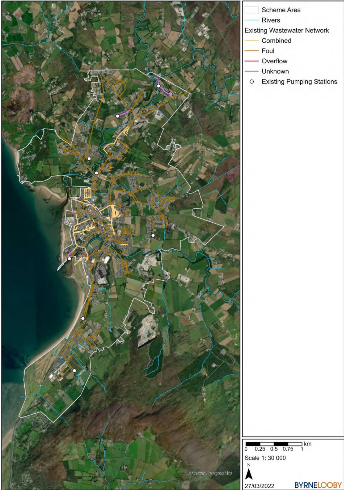
Figure 3.2 Existing Wastewater Network
