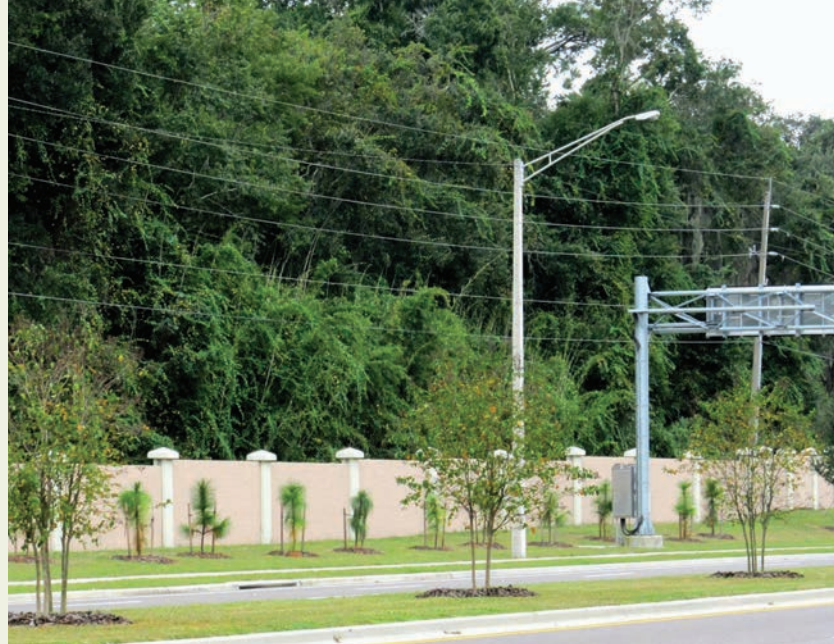
Plan ahead! These longleaf pines ( Pinus palustris ) were planted too close to overhead wires. The best case scenario as they mature is that only half of their branches will be pruned away. Worst case is that they'll be removed entirely and that people in charge of making decisions on street trees will decide that native trees don't do well in urban environments.
