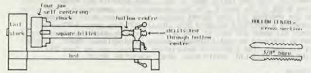
I bore square billets holding them in a four jaw self centering chuck ( see Comm 958 ). At the tailstock end I use a hollow-or 'ring nose' centre. This is basically a steel tube with the front edge sharpened. It is tightened into the end of the wood in the same way as a normal pointed centre and it cuts a circle into it, leaving the actual centre of the wood free for boring.
