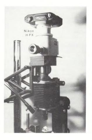
Figure 3 (at left). The Nikon HFX unit mounted on the compound microscope. The umbilical wiring to the HFX unit and the control box do not show. Note adjustable specimen pedestal at bottom, and the fiber optics light source coming in from the left.
