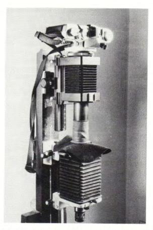
Figure 2. SLR setup for photographing through the compound microscope.
