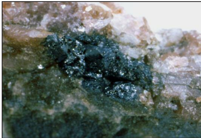
Långbanite - (\text{Mn}^{2+}, \text{Ca}) (\text{Mn}^{3+}, \text{Fe}^{3+})_9 \text{Sb}^{5+} [\text{O}_8|\text{SiO}_4]_2 Långbanite grain is 5mm across, in rhodonite (?) mix. Locality - Gozaisho mine in Fukushima, Japan. Excalibur Mineral Corp. specimen. Photo by Dr. Jeff Weismann
