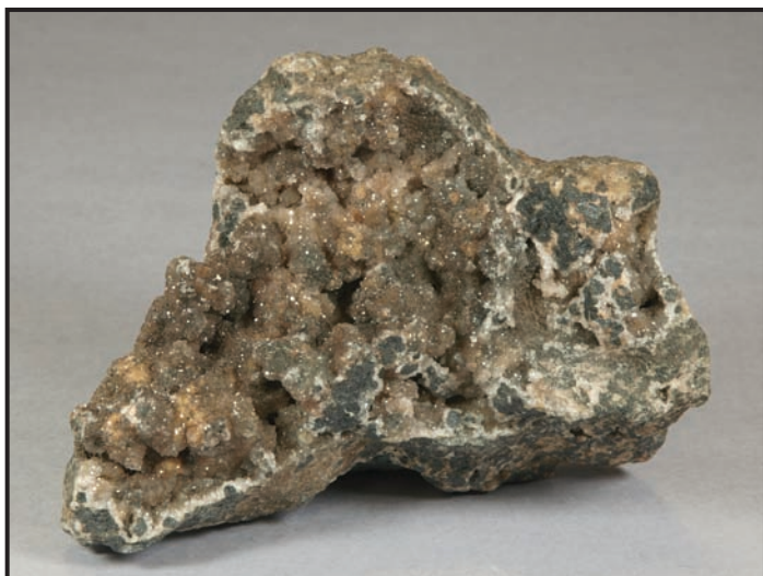
Figure 5. Solution vugs lined with quartz in franklinite-willemite-calcite zinc ore from Sterling Hill. Specimen size is 4\frac{1}{2} \times 3\frac{1}{4} \times 2 inches ( 11.5 \times 8 \times 5 cm). Earl R. Verbeek photo.
