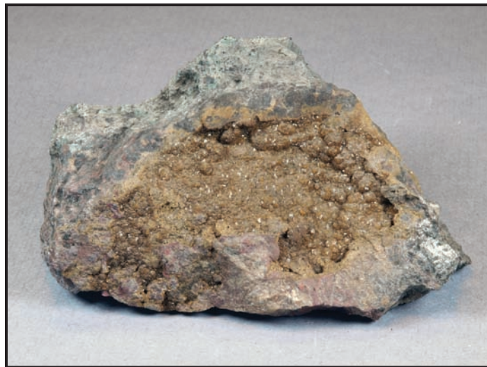
Figure 4. Rhombohedral crystals of brown siderite in a shallow solution vug in ore from Sterling Hill. Bearing catalog no. 407, this specimen is on display in the Franklin Mineral Museum; it measures 4\frac{1}{4} \times 2\frac{1}{4} \times 2 inches ( 11 \times 7 \times 5 cm). Earl R. Verbeek photo.
