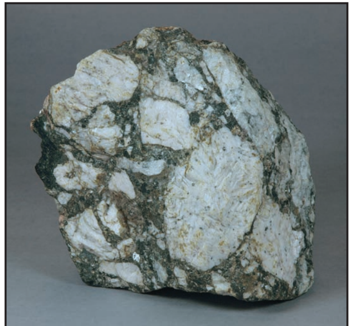
Figure 16. Solution-collapse breccia from 700 level, Sterling mine, consisting of clasts of Franklin Marble in graphitic matrix, cemented by later carbonate. The graphite explains the dark matrix color of most solution-collapse breccia derived from the Franklin Marble. Specimen size is 5 × 4.9 × 2.8 inches (13 × 12.5 × 7 cm). Earl R. Verbeek specimen and photo.
