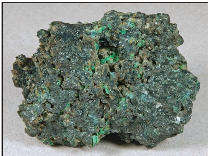
Figure 2. Chalcocite, partly altered to green, secondary copper minerals, in a vuggy mass of franklinite from which the calcite had previously been dissolved. Though both the franklinite and chalcocite are black, and thus not readily distinguished from each other in the photo, the franklinite has bright metallic luster and the chalcocite is dull. Originally in the John Kolic collection, this specimen is from Sterling Hill and measures 3 \times 2\frac{1}{4} \times 1\frac{1}{2} inches ( 7.5 \times 5.5 \times 3.5 cm); it is now specimen no. SHMM-2254 of the Sterling Hill Mining Museum. Liz Schneider photo.
