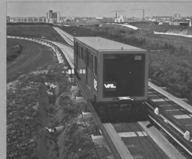
Fully Automatic VAL Urban Transit System in Lille, one of several experimental systems.
