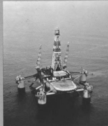
Neptune Offshore Drilling Platform in the North Sea: The floating platform for offshore oil prospecting has an electric power plant and living quarters for some 60 people.
