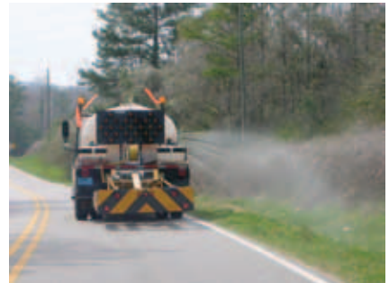
Roadside sprayers can treat invasives along highways.
