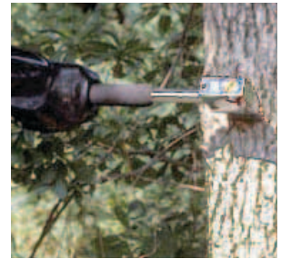
Hypo Hatchet® Tree Injector.
