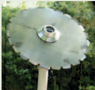
Brushsaw blade with chainsaw-like teeth.
