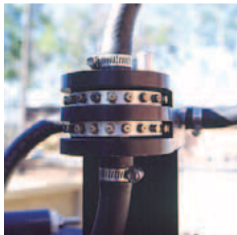
Radiarc® Sprayer 22-tip head.
