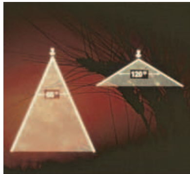
Nozzle spray angles of 65 and 120 degrees.
