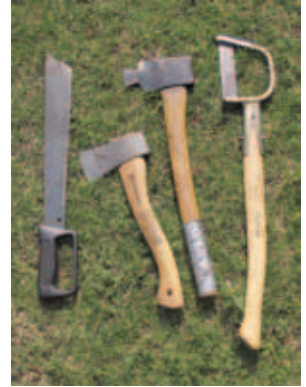
Cutting tools for hack-and-squirt treatment.
