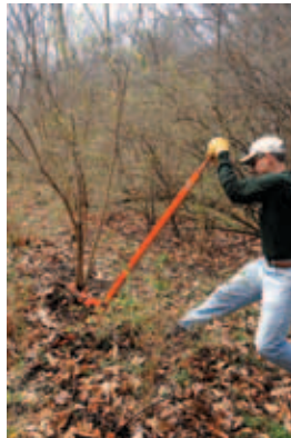
A shrub wrench enhances human strength by the lever.
