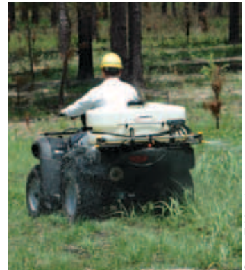
ATV mounted sprayer with a boom.
