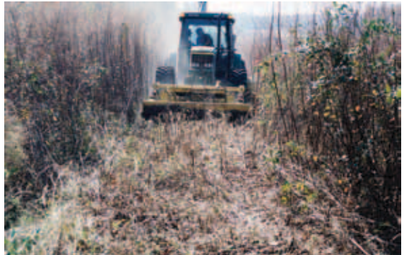
Wetblade brush mower applies herbicide while cutting.
