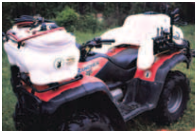
ATV mounted sprayer with front and rear tanks.
