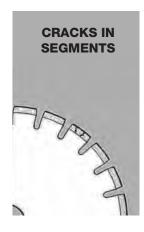
1. The blade is too hard for the material being cut.
