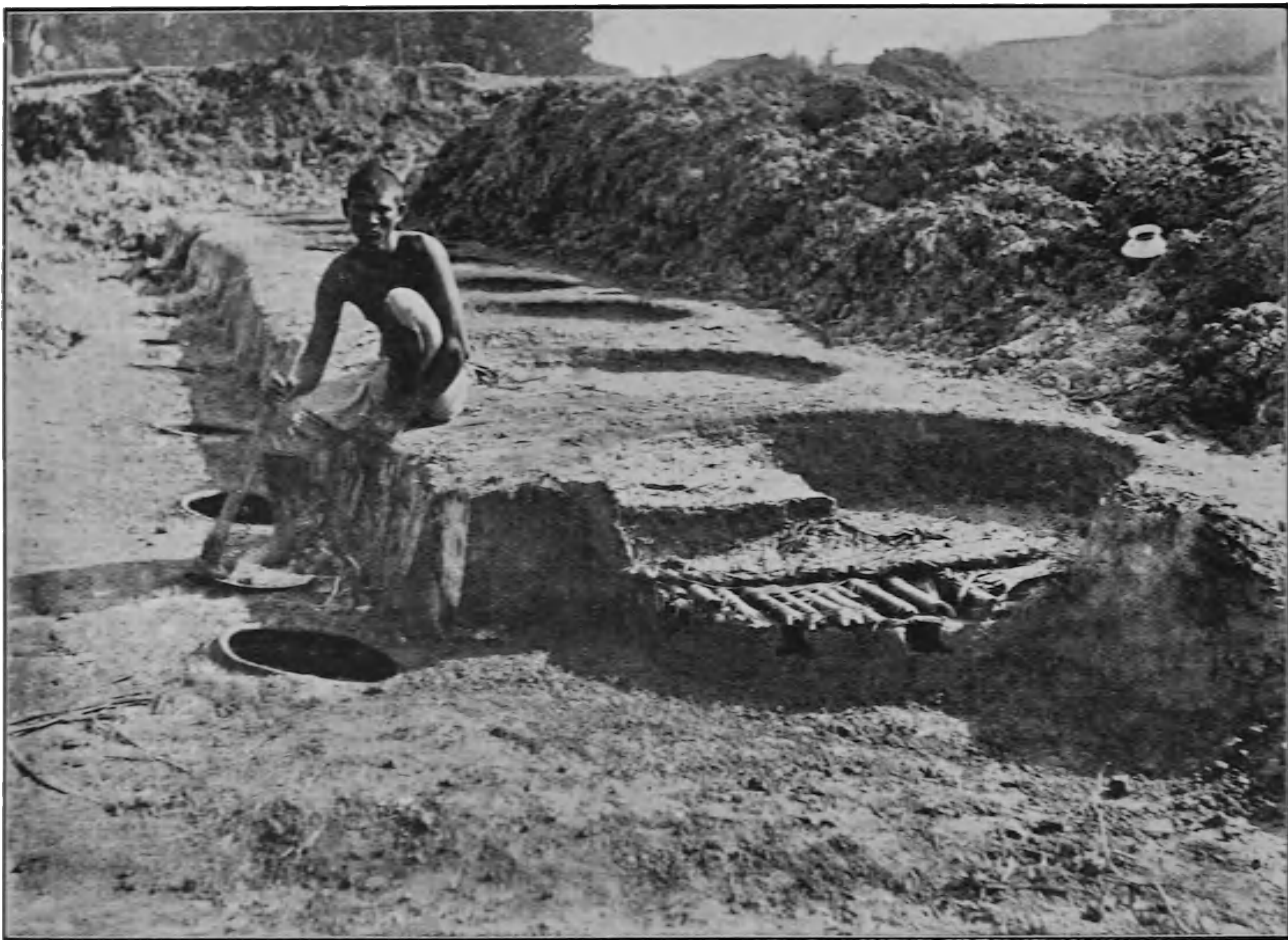
FIG. 3. Percolators for Extracting Indian Crude Saltpetre.
