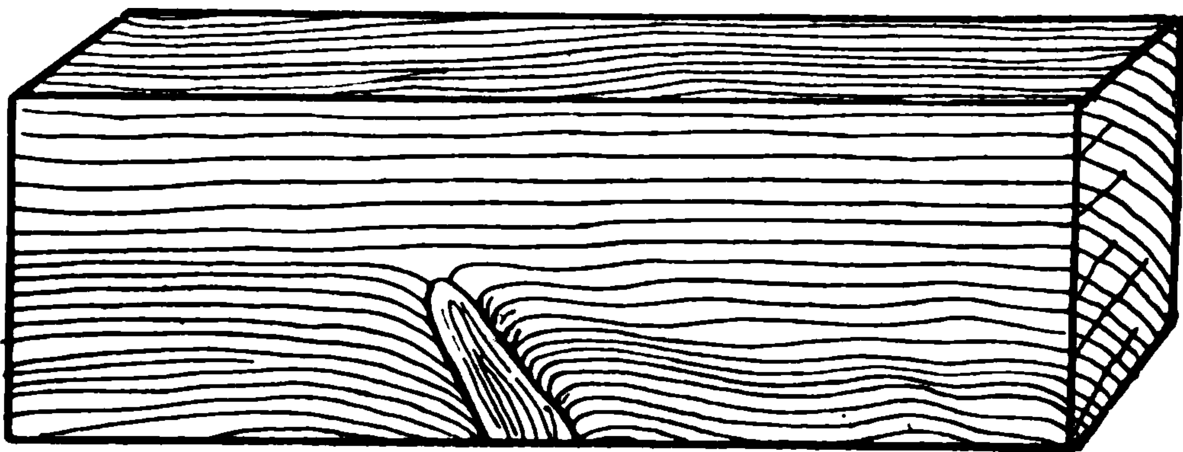
FIG. 49.--Showing risk of knots on underside of loaded beams.
