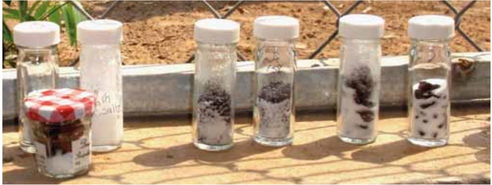
Salt can also be used in a crude test for moisture content. Quarter fill a small glass jar with very dry table salt, add about an equal volume of seeds and shake. If the salt forms clumps, the eRH is higher than 70%. If the salt remains free flowing, then the seeds can be stored, at least in the short term.
