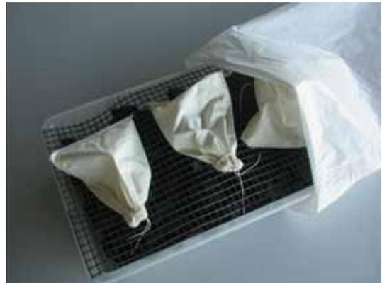
Charcoal in a sealed container or in sealed bags can be used as a natural desiccant. (Photo: K. Mistry)
