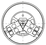
Single-phase capacitor with d = 60/70 mm Spring tension terminal AKD 25/2 for 2 \times 6 mm 2
