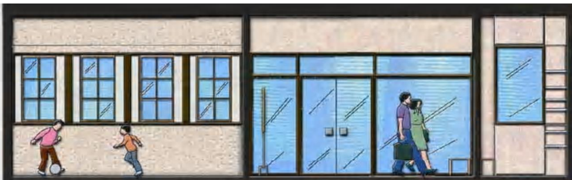
Figure 39 Adding people on interior elevation drawings gives a relative sense of object heights
