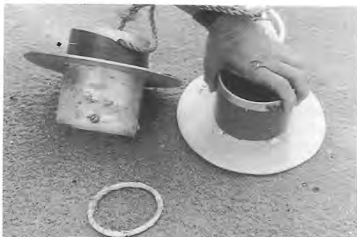
FIG.6. 'Depth rings' being placed in the bed to measure depth of sediment disturbance by scallop dredges.
