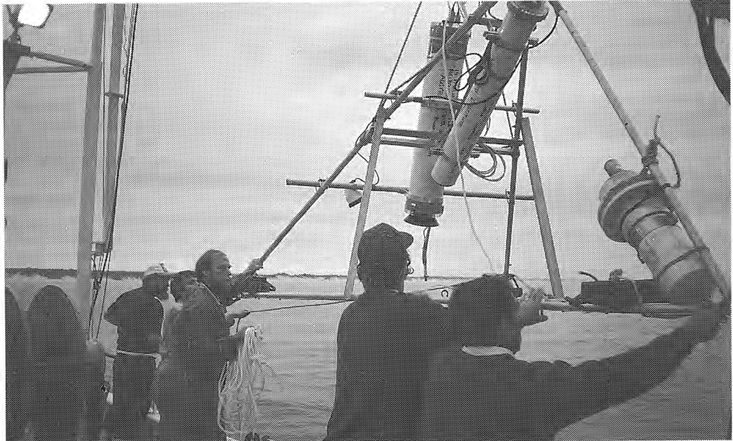
FIG.3. In situ sediment transport unit (SEDCAM). The underwater video camera and the sediment sensor electronics are within the large housing. The smaller housing contains a battery power supply for the equipment and underwater lights. An acoustic pinger (foreground) is included to assist retrieval, if the frame was accidentally moved by a fishing boat.
