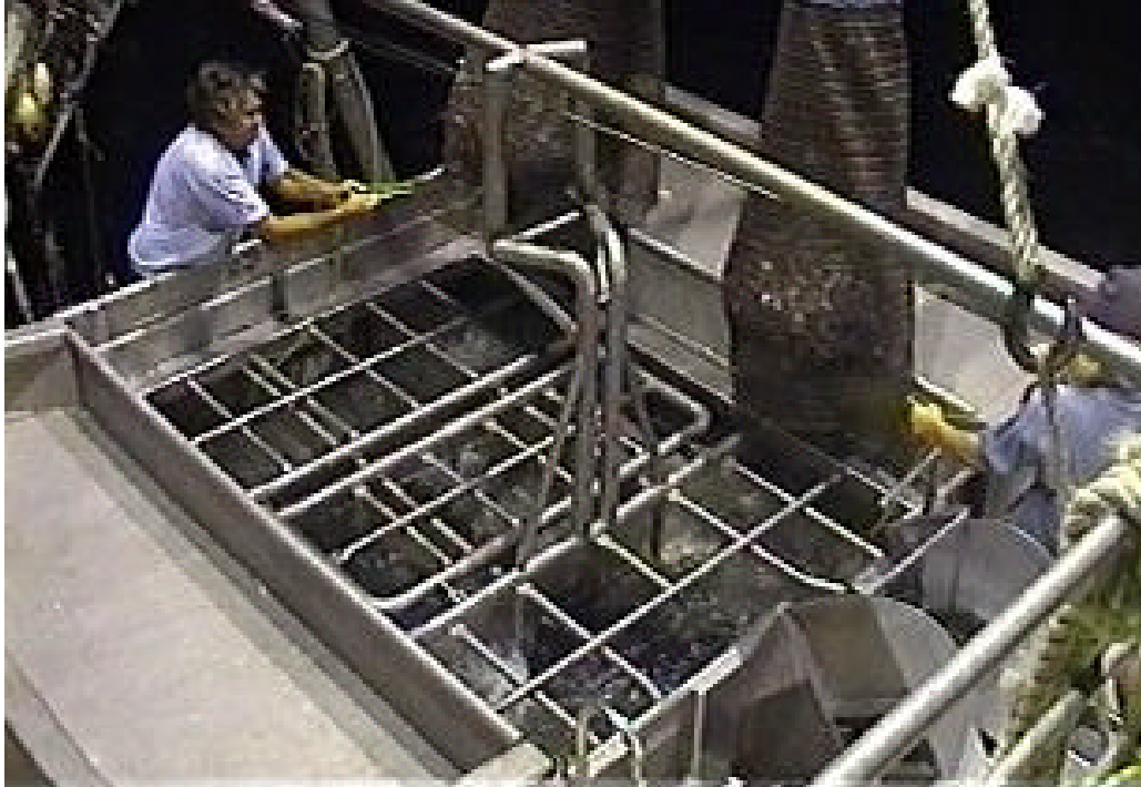
Figure 1: The catch is emptied into a Hopper full of flow-through seawater and then transferred via conveyors for processing with minimal physical handling.
