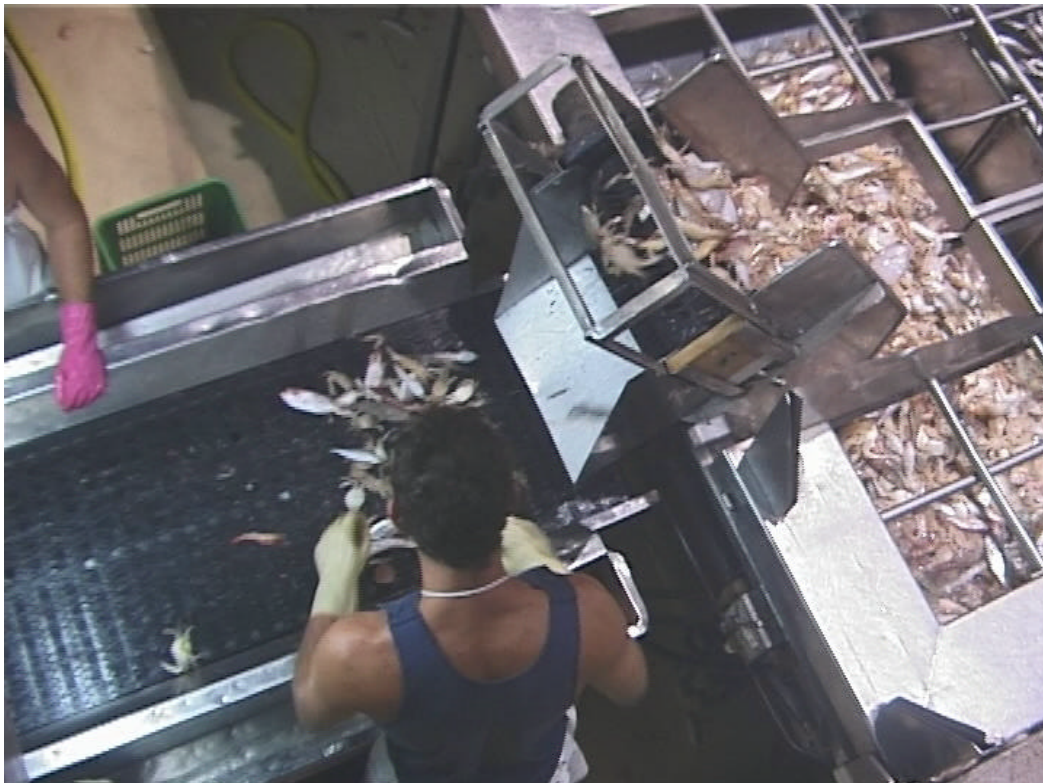
Figure 2: Catch is removed from the Hopper via elevator conveyors onto a sorting conveyor.
