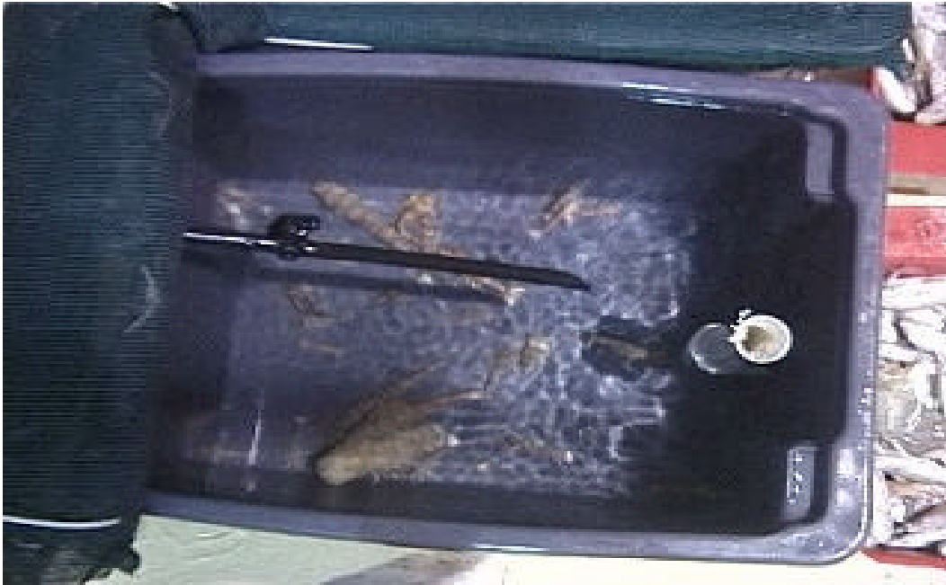
Figure 7: Flow-through tanks used for onboard survival experiments. Each tank had an individual feed line and control tap to regulate water flow rate.
